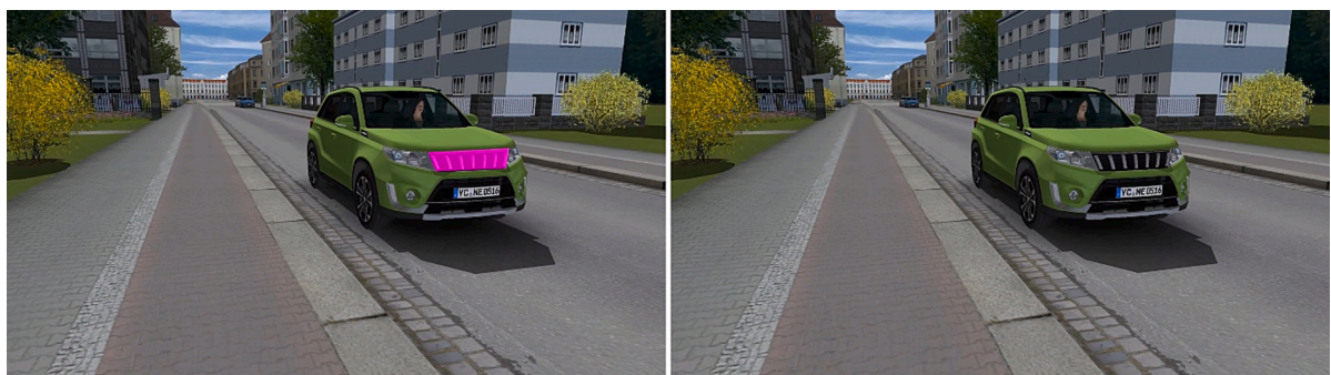
Fig. 1. Screenshot of a decelerating vehicle (left: equipped with an FBL; right: not equipped with an FBL).
